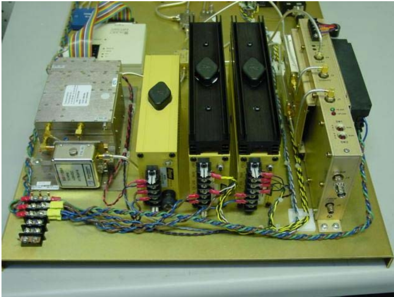
Receiver Plate Stalo (w/ 10 MHz ref source), DC Power Supplies and IFD
