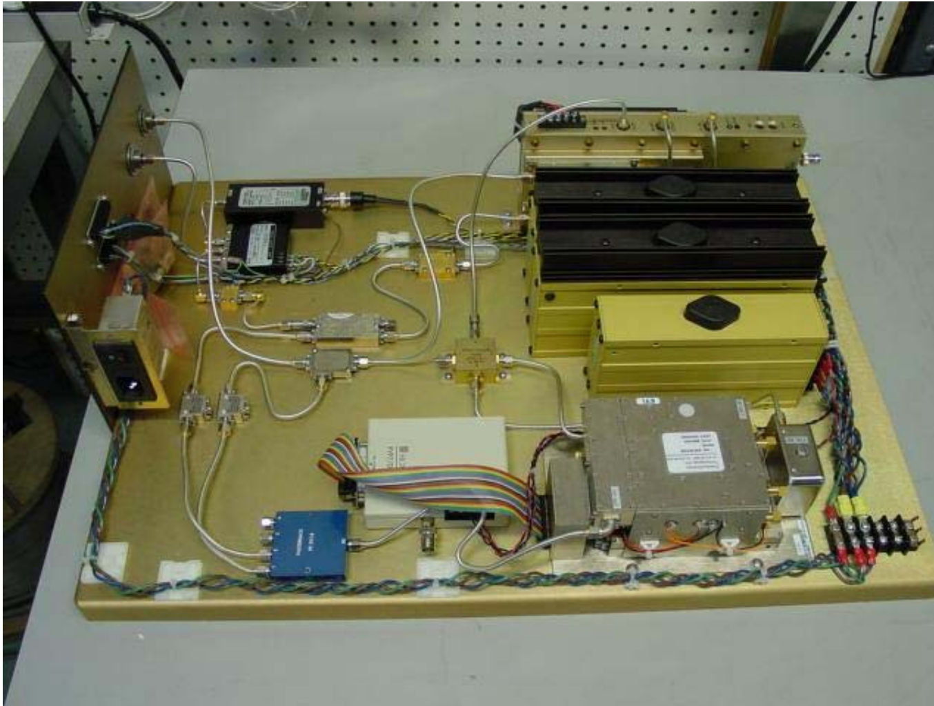
Receiver Plate Perspective showing RF component interconnection.
