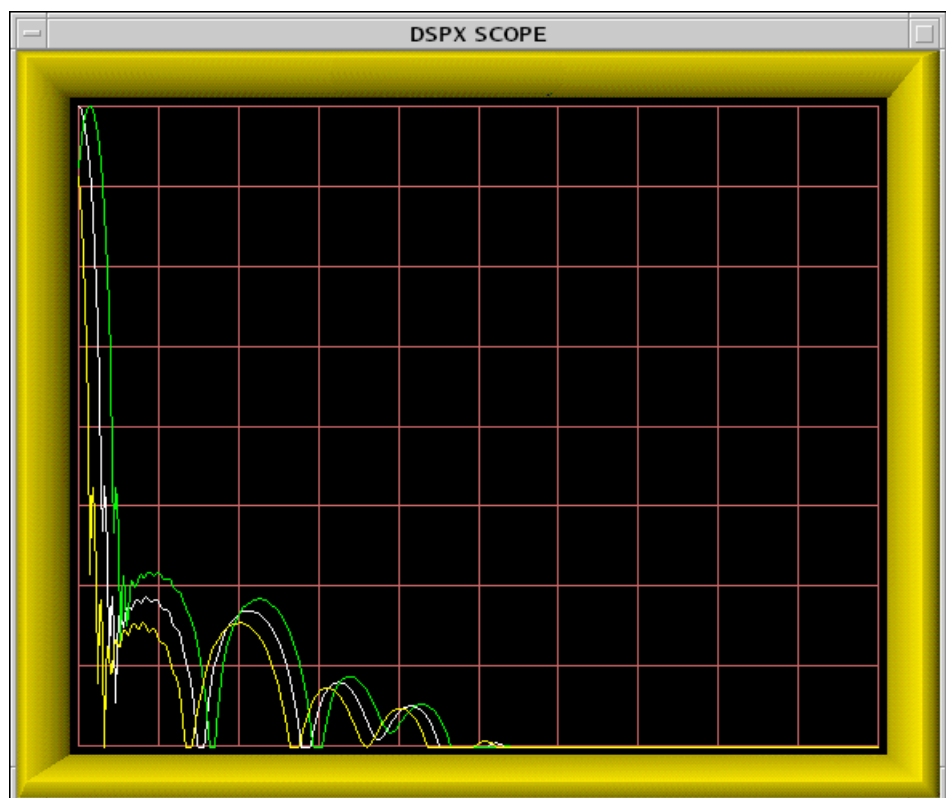
Figure 32 Ambiguity Diagram of a Compressed Tx Pulse
