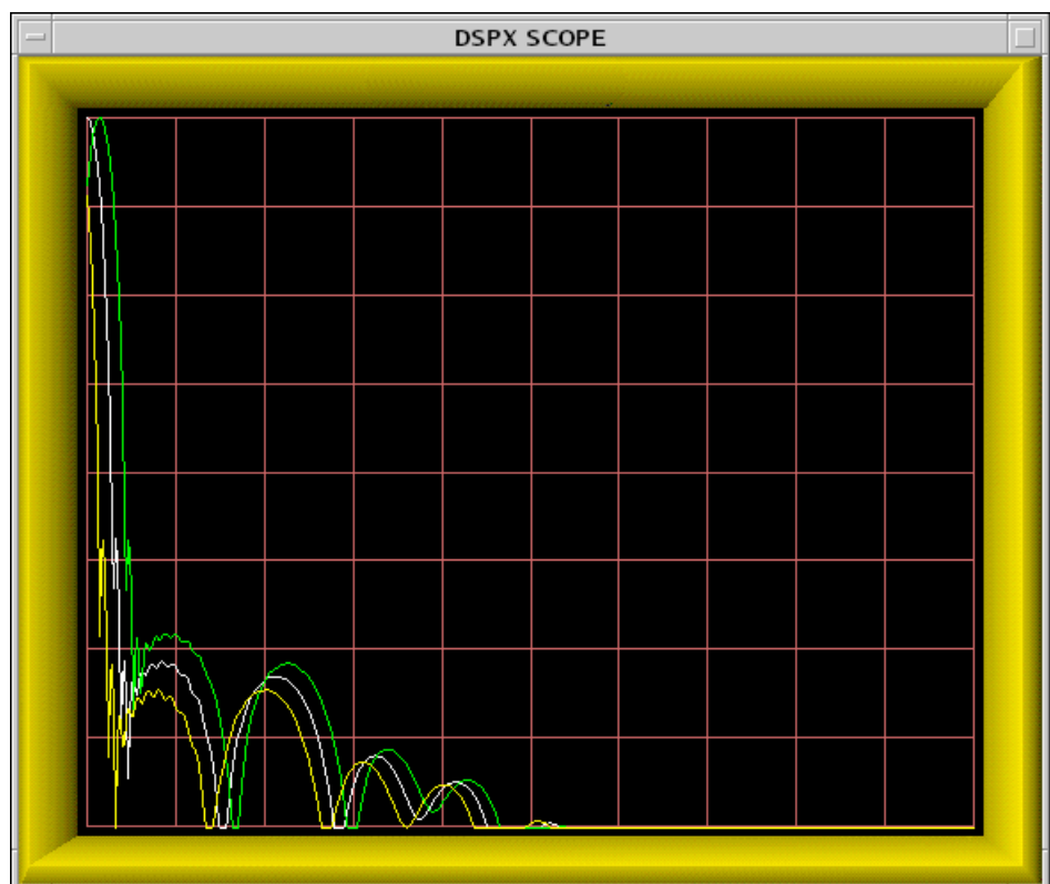
Figure 32 Ambiguity Diagram of a Compressed Tx Pulse
