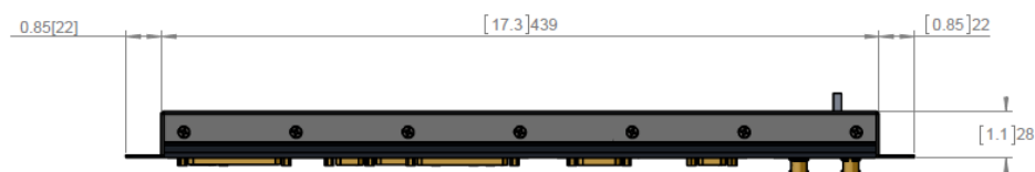
Figure 76 RCP902 WSR98D Top Panel Dimensions
