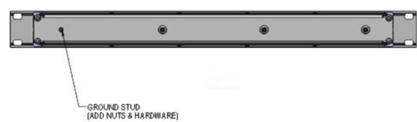
Figure 73 RCP903 Back Panel Dimensions
